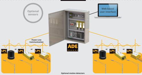
The TLACS is an intelligent addressable lighting control system using advanced power line communication to control and monitor the lighting system status. Already used in over 100 infrastructures worldwide, TLACS-A is a simplified version adapted for the specifics needs of outdoor area lighting. It uses the wires that feed the luminaires to achieve two-way communication.
