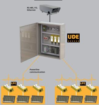
The Underpass Dimming Enclosure (UDE) is the main controller that interfaces each luminaire individually using powerline communication via 0-10V, LPC (Local Product Controller) is installed in every luminaire. This means, no control wires to install for a quick and seamless lighting system upgrade.
