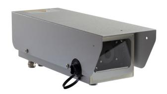
The LCAM uses a specially designed, highly light-sensitive photocell filtered to provide a spectral response close to the average human eye for optimal performance. The light receptor measures the average luminance over a scalable range of 0 - 10,000 cd/m² within an opening angle subtending 20° as recommended by CIE 88:2004 and RP-8-18.
